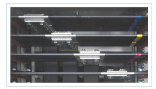
Safer busbars – Busbars in Ti range have higher clearances than those provided by global switchboard standards (25mm - Ph to Ph and 19mm - Ph to N/E) offering superior safety.
